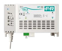
**OPT-MBJ optical receiver** with one wideband RF output for receiving TV+SAT signals distributed over a single fiber. Optical input range of **0 to -15dBm**; optical window of operation 1270-1610nm. (dimensions 135x82x39mm)
